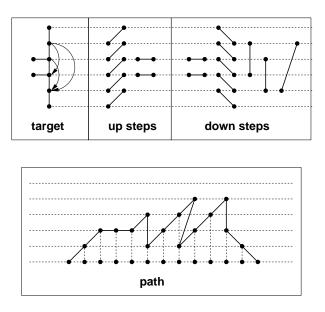
Figure 6.3: Two-dimensional lattice path representation on the graph  $\Gamma_{\mathbf{M}}$ ,  $\mathbf{M} = (2, 1, 0)$  of the  $A_3$  case. We have indicated the "up" steps (i.e. away from the root) and the "down" steps (towards the root).
