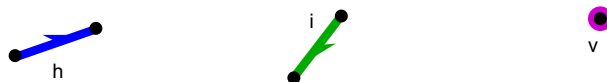
Figure 4: Pictograph representation of a half-edge h directed toward a vertex v , and a half-edge h' directed away from v .
