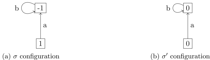
Figure 8: A graph with \sigma given on the left and \sigma' on the right. Consider \sigma \xrightarrow[r]{\partial} \sigma' : the unique transitory vertex is the bottom one since the top one is not active. Then \{a\} is a guiding tree for that routing and there is a legal routing sequence with routing vector a . Consider now \sigma \xrightarrow[r]{\partial} \sigma' . Both vertices are transitory, but there is no guiding tree for a + b . One can easily check that there is no legal routing sequence from \sigma with routing vector a + b .
